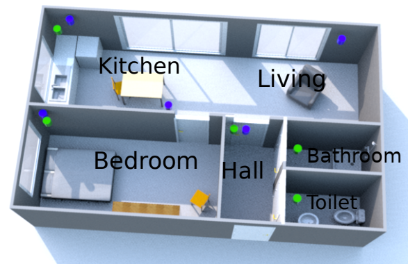
Figure 2. Simplified overview of location 1. The locations of the five motion sensors (green cylinders) and cameras (purple cylinders) are shown.
